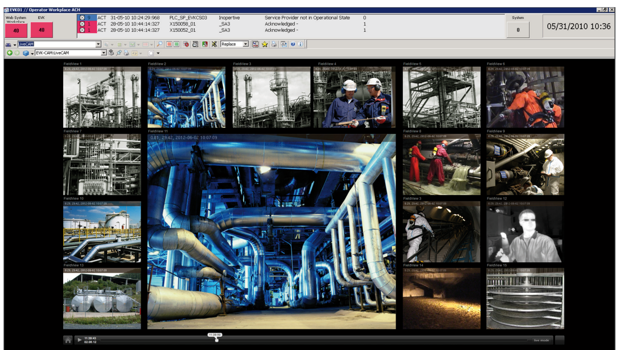
Figure 3: The figure shows a visualization of a 15-stream-video-wall in the process control system 800XA from ABB.
