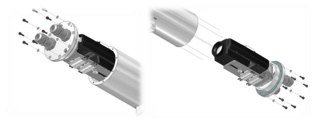
Fig. 6-3: Opening the ExCam T08-VAx.x.x. camera
