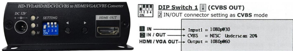
Figure.5.1 – Setting of the DIP Switch Videoconverter
