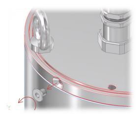
Fig. 6-5: Removing the countersunk screw, type T08-TNXCD
