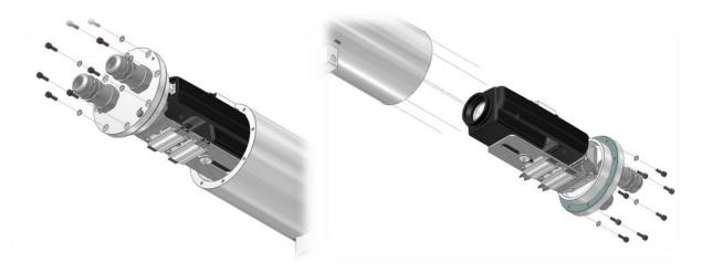
Fig. 6-3: Opening the ExCam T08-VAx.x.x.x camera
