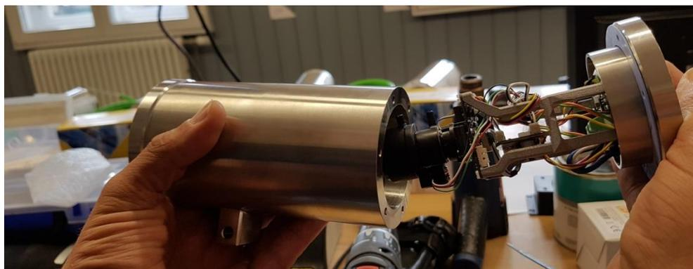
Figure 5.3 removing the camera
