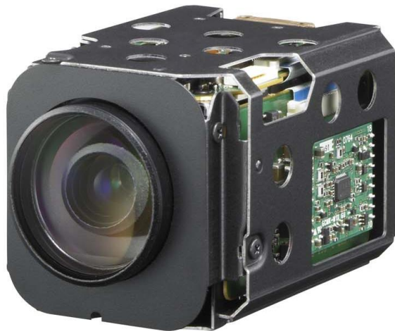
Figure 4.9 RoughCam® niteZoom – lens and sensor board
