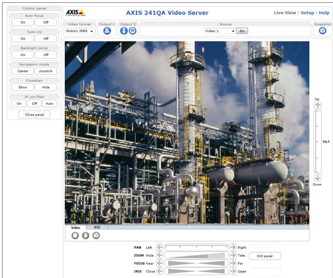
Figure 4.8 Control and visualization via a video server
